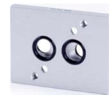
ZPN 1/4-1/2 Adapter plate to assemble a 1/2" NAMUR-valve to an actuator with 1/2" NAMUR-interface.
