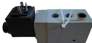
Aluminum – EMATAL valve after 720 hours in salt spray chamber
