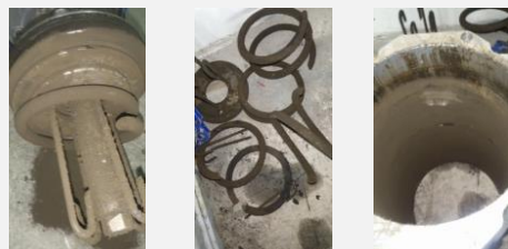
Broken springs in single-acting actuators in a paper mill.
